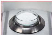
Numerical values fluctuate due to electrically charged powder in a Petri dish
